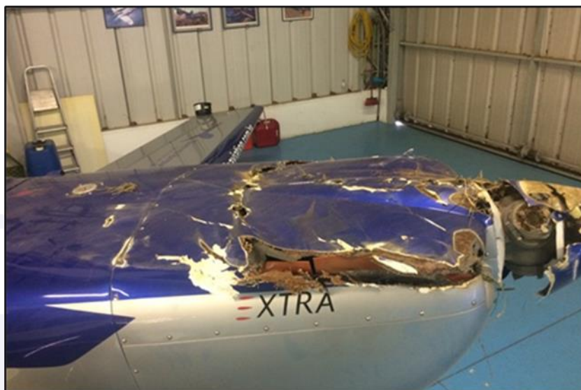
Figure 2 - Engine hood, spinner and propeller damage.
