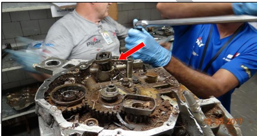
9 10 Figure 21 – Gears of the accessory box. The arrow indicates misalignment of the drive 11 gear of the right magneto.
