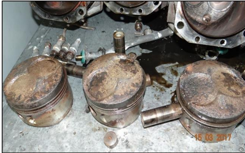
3 4 Figure 26 - View of the pistons 1, 2 and 3, with normal working color.
