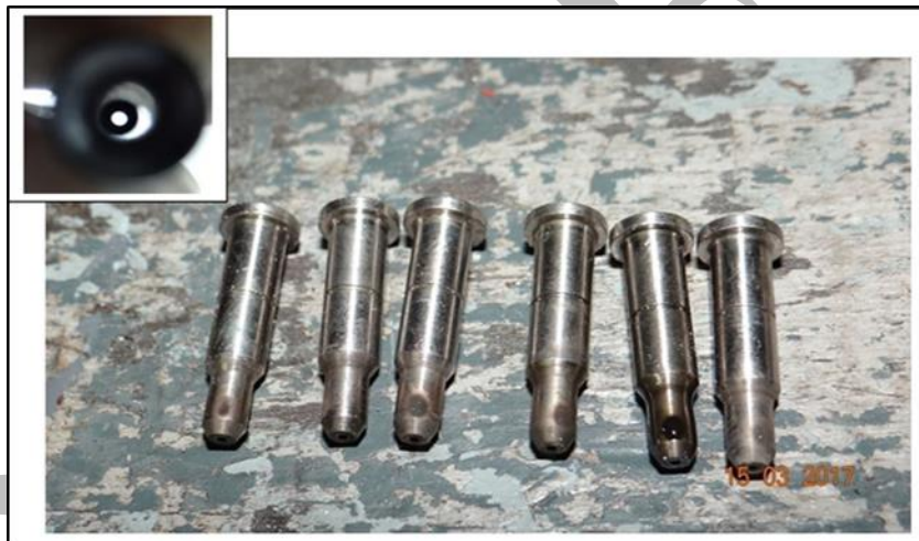
7 8 Figure 12 - View of the nozzles. Highlights the clearing.
