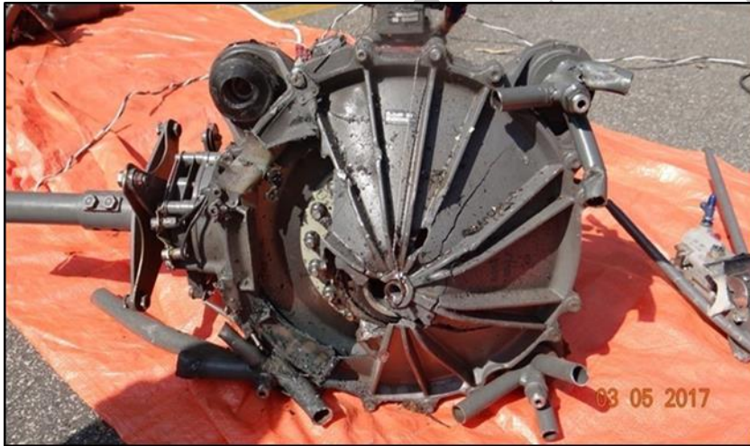
5 6 Figure 36 - View of the transmission case crankcase fracture.
