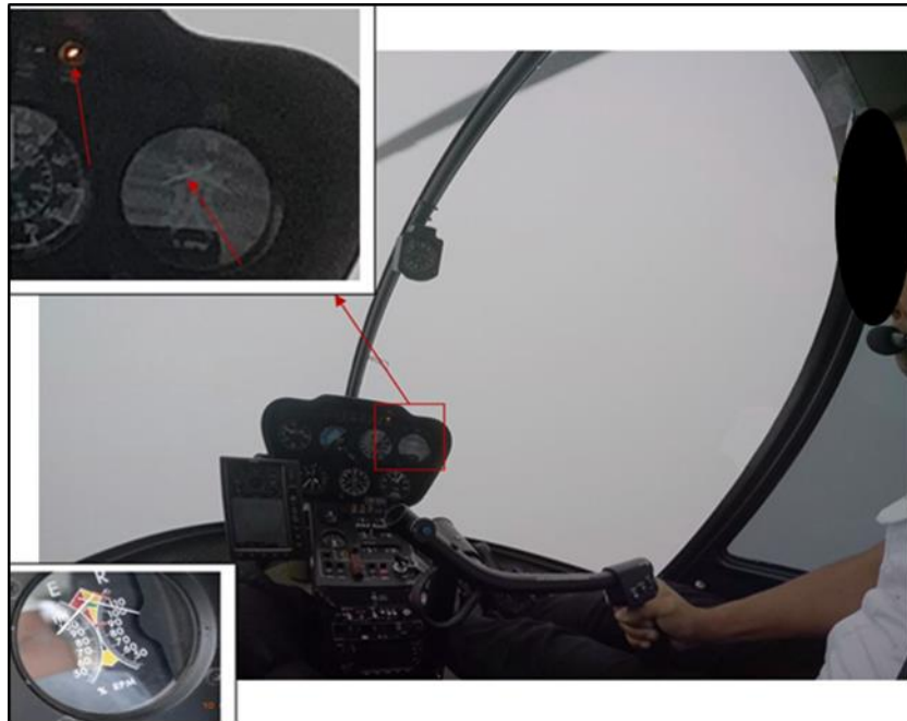
Figure 47 - Low RPM Main Rotor Indicator Light. In the lower highlight, an indicator similar to that of the aircraft. In the top highlight, indication that the engine was powered.
