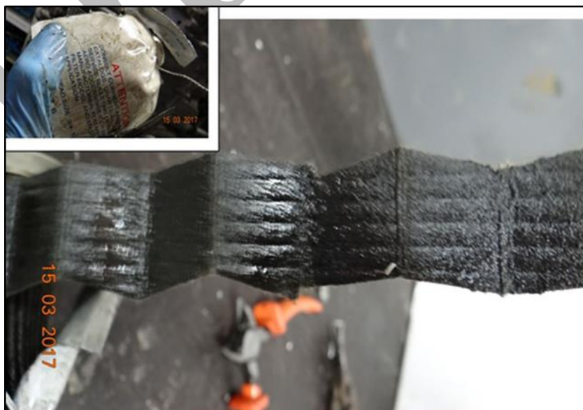
7 8 Figure 19 – Oil Filtering element with no filings. Highlighted the oil filter before opening.
