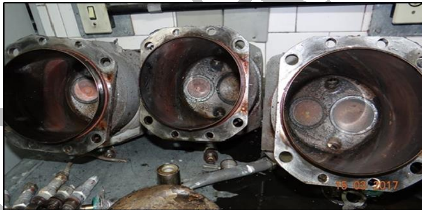
13 14 Figure 24 - View of cylinders 1, 2 and 3, with no operational damage.
