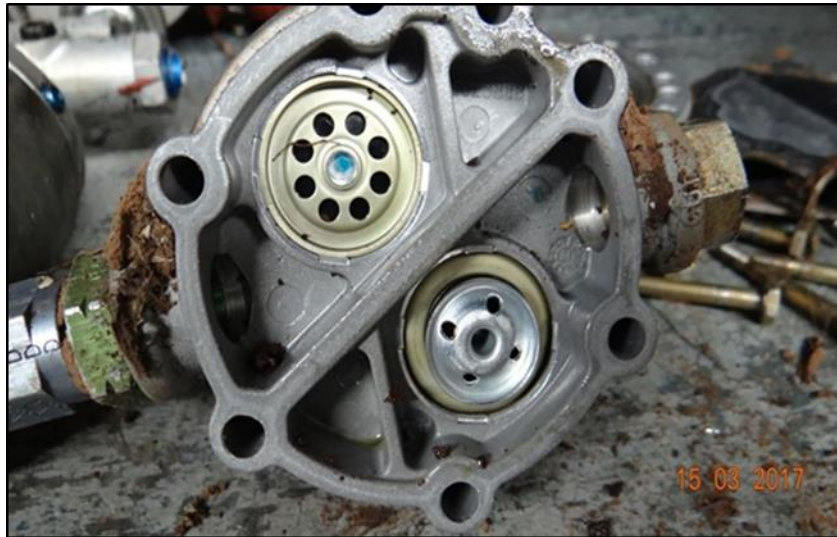
1 2 Figure 17 - View of the interior of the fuel pump, showing its valves.
