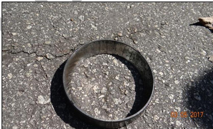
9 10 Figure 40 - Transmission case lower bearing outer race, undamaged.
