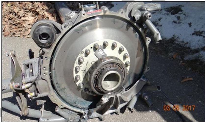
7 8 Figure 39 - Bottom view of the rack and bearing of the transmission box.
