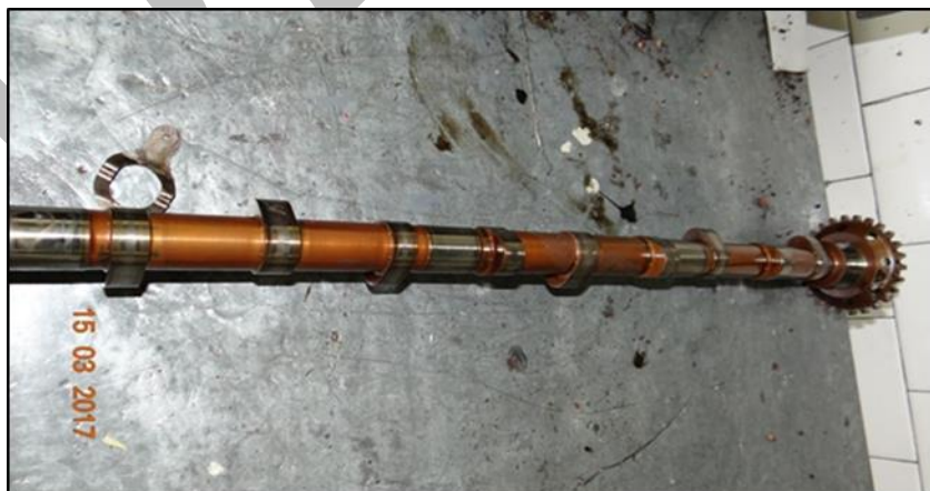
8 9 Figure 28 - Overview of the engine valve control shaft.
