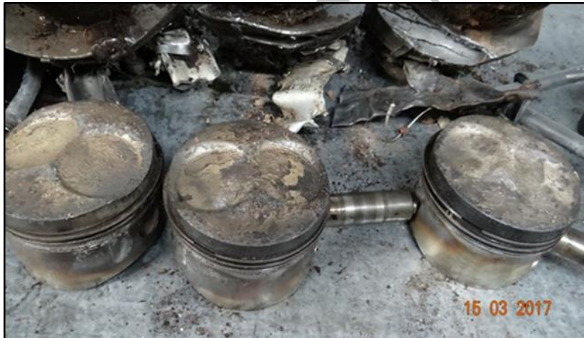
5 6 Figure 27 - View of the pistons 4, 5 and 6, with normal working color.
