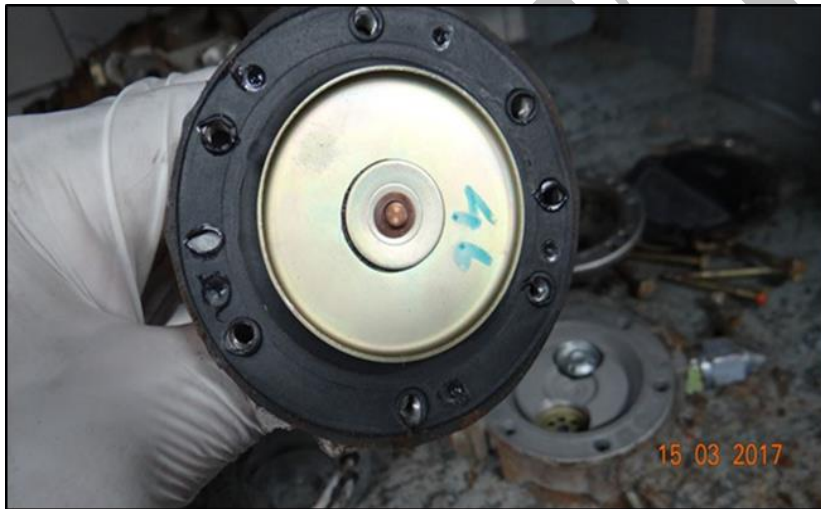
3 4 Figure 18 - Clean fuel pump diaphragm view.
