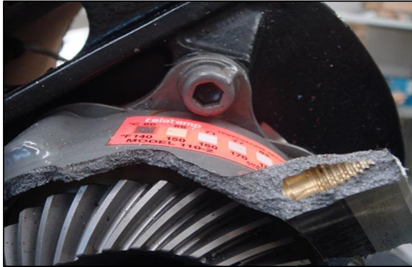
Figure 8 - Surface of fracture with aspect of overload.
