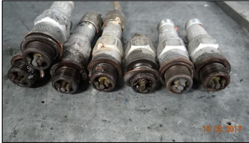
4 5 Figure 11 - Spark plugs with normal operating color.
