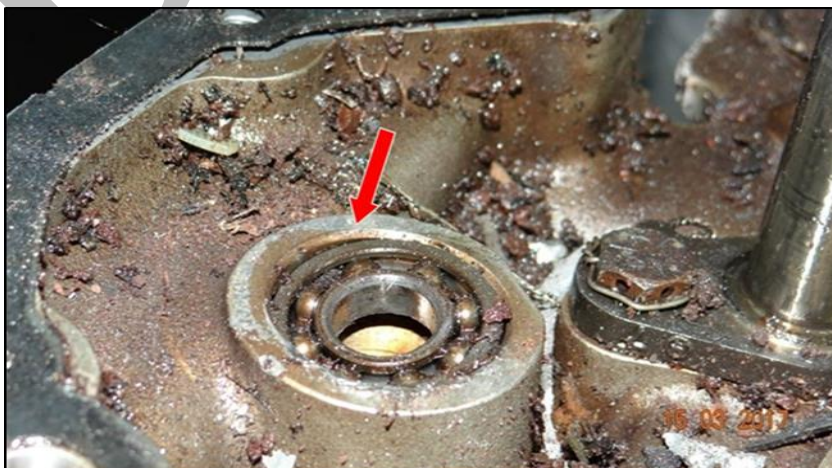
13 14 Figure 22 - Misalignment in the drive gear bearing of the right magneto.
