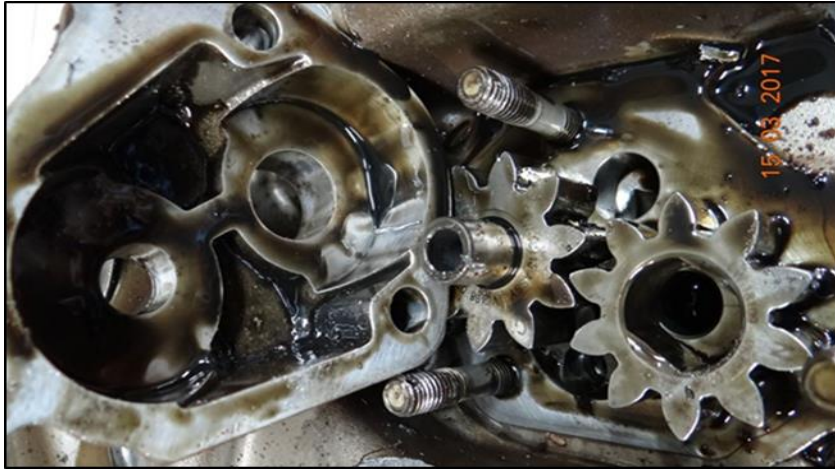
4 5 Figure 20 - Gears and housing of the engine oil pump without scratches.
