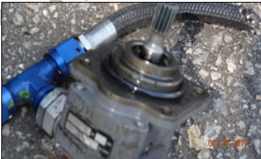
9 10 Figure 37 - Main gearbox hydraulic pump.
