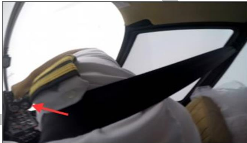
8 9 Figure 67 – 18:30:18 (UTC), indication that the engine was still running.
