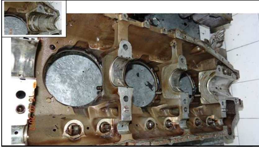
4 5 6 Figure 32 - View of the right semi-engine housing and of the connecting rod in good condition.
