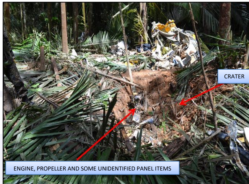
Figure 5 - Crater and place where the engine and the propeller were buried, plus some unidentified panel items.
