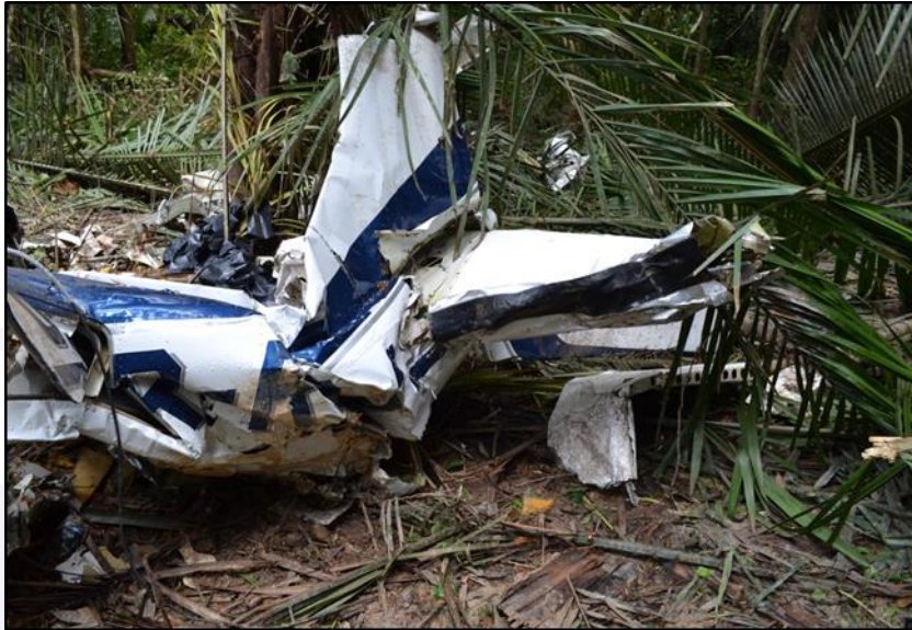
Figure 7 - Tail of the aircraft without rudder and elevator. The violence of the impact against the ground can be identified by the kneading and twisting of part of the fuselage observed in the photo.
