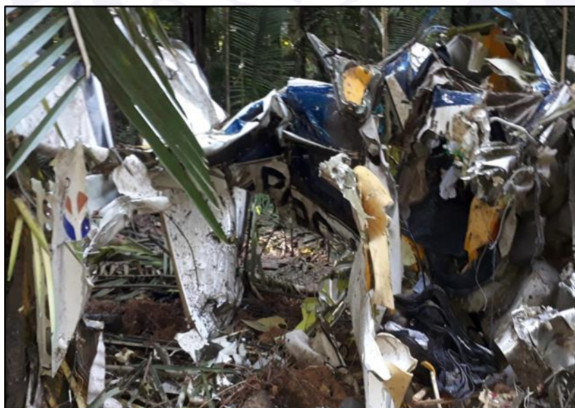
Figure 6 - Position of the aircraft after the total stop. Without wings and with the cabin destroyed.
