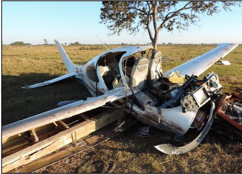
Figure 3 - General view of the wreckage. Cabin and right wing destroyed.
