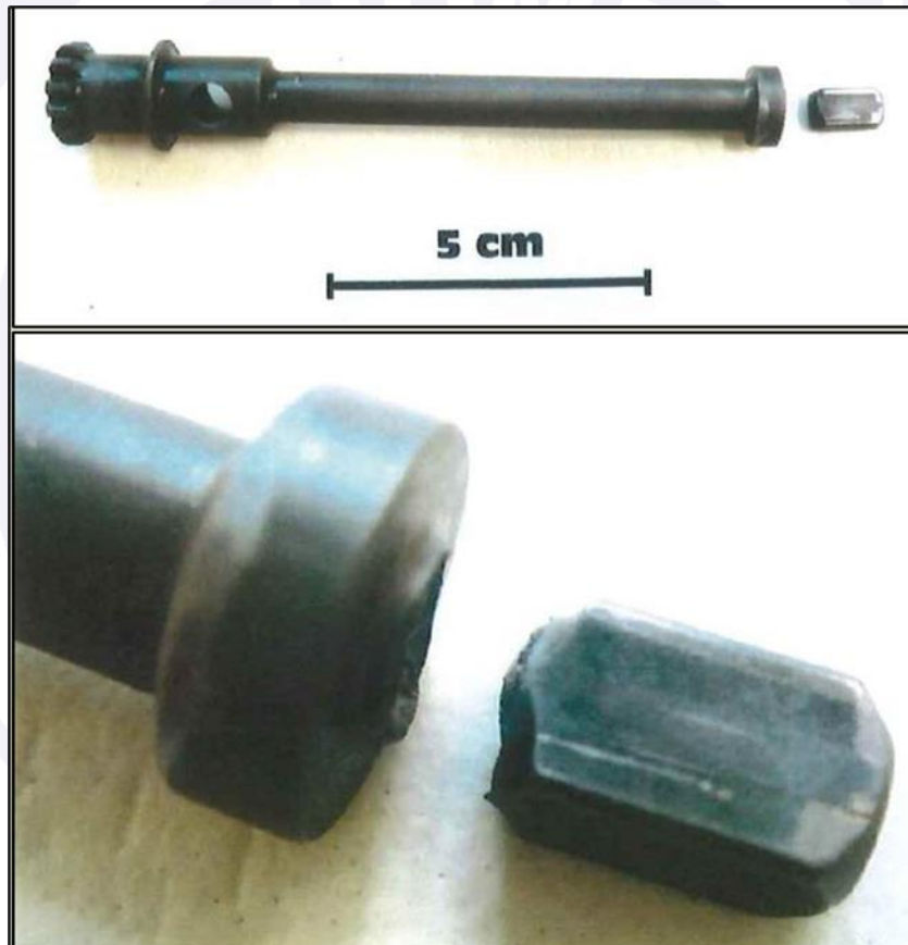
Figure 9 - Engine fuel pump drive shaft with fracture at its end.
