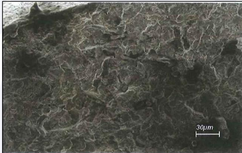
Figure 11 – Electro micrograph showing the fragile aspect of the fracture, with cleavage and intergranular mechanisms.
