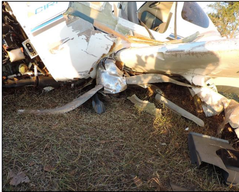
Figure 5 - Propeller set detached and found under the fuselage, with folding blades.
