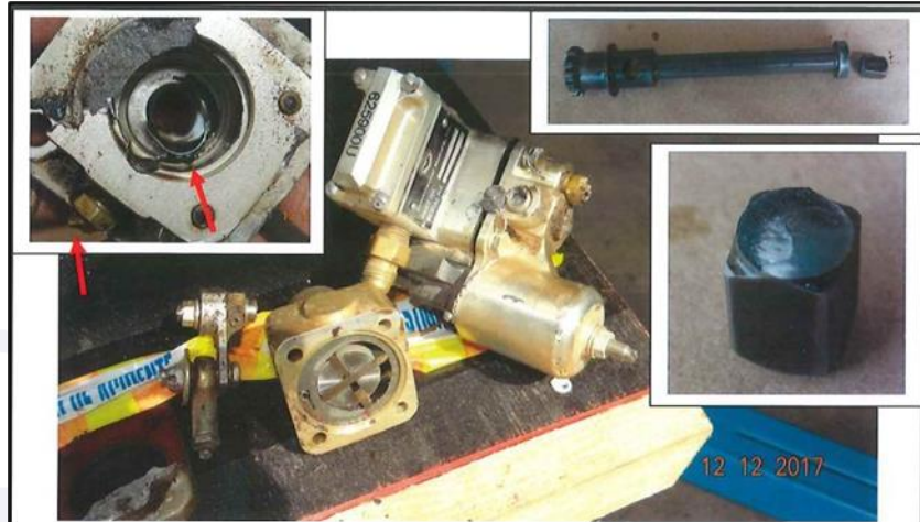
Figure 8 - General view of the fuel pump. Highlighted on the right are photos of the drive shaft and the fracture surface at its end. Left highlight shows observed damage to pump retainer and connection.
