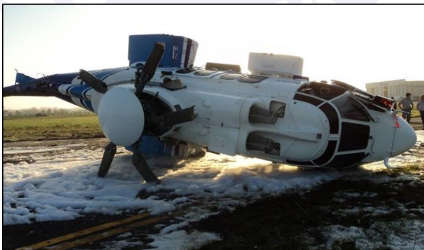
Figure 2 - Aircraft tilted to the right and impact of the main rotor against the ground.
