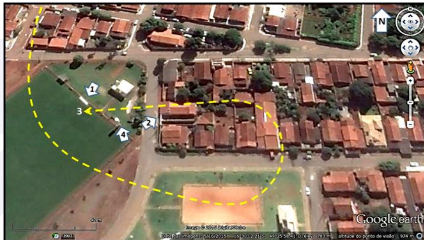
Figure 5 - The dashed line in yellow indicates the approximate trajectory described by the pilot. "1" - indicates the goal; "2" - indicates the gate hit by fragments of the goal; "3" - indicates the final stop position of the aircraft; and "4" - indicates a water tank by the side of the field.
