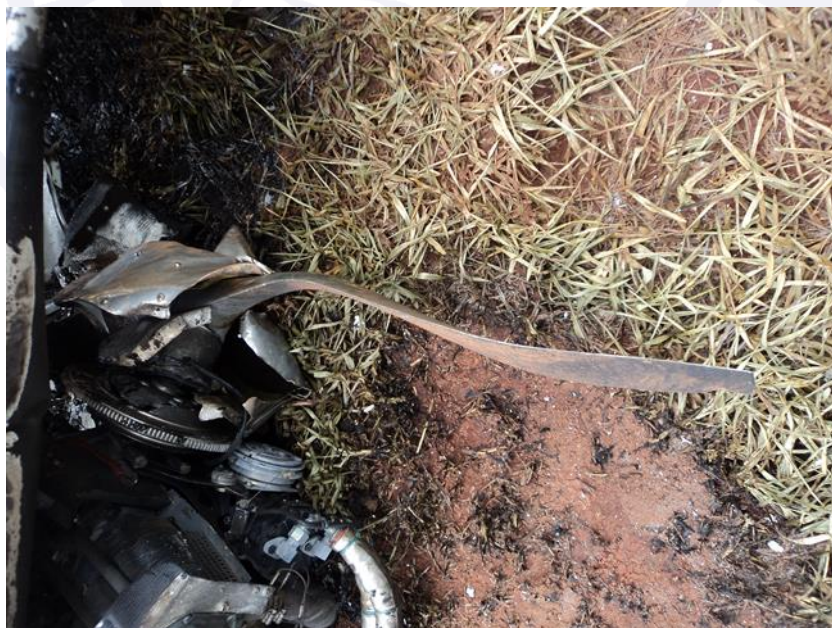
Figure 5 - Deformation in one of the aircraft propeller blades with evidence of wide angle impact and against soft ground.
