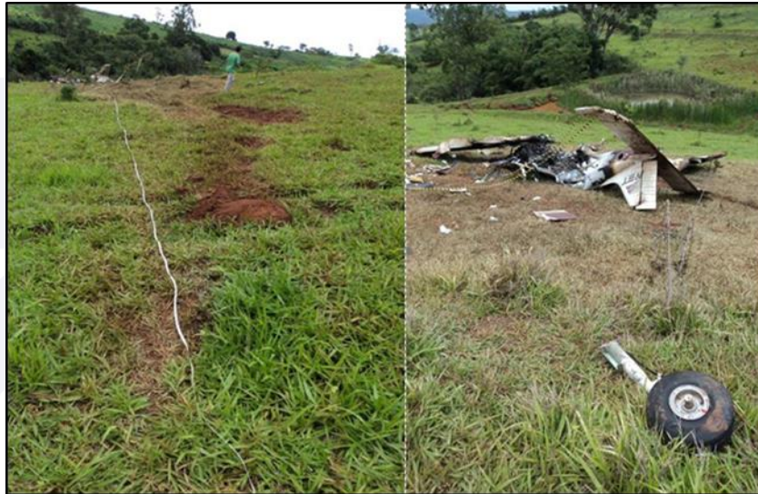
Figure 4 - Trajectory of the aircraft after the collision against the ground, leg of the landing gear that detached from the aircraft after the impact (foreground) and concentration of the wreckage (background).
