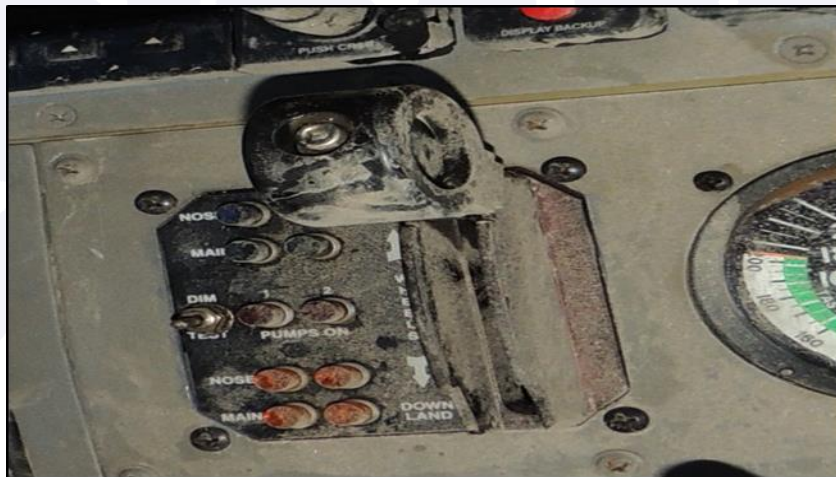
Figure 8 - Position of the landing gear control.
