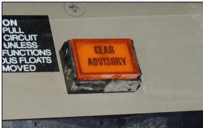
Figure 4 - Gear Advisory button installed on the PR-MPE aircraft.
