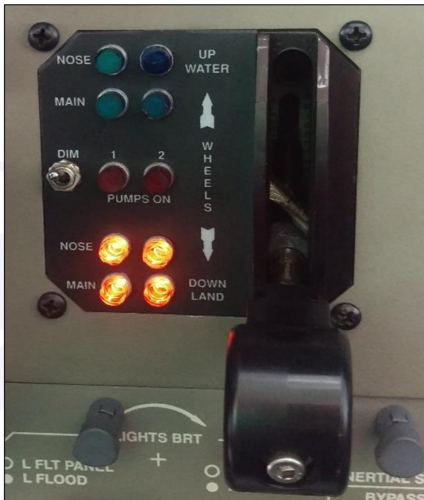
Figure 3 - Amphibian landing gear control and light system.
