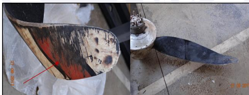
Figure 13 - Scratches and kneading of propeller blades.
