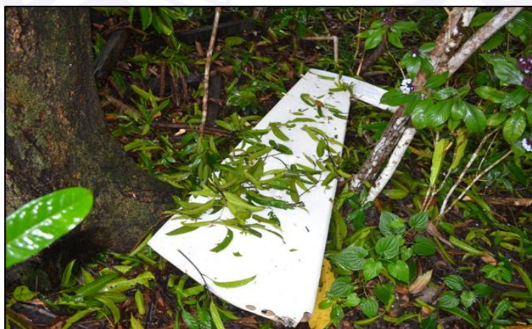
Figure 2 - Left elevator found near the first impact site.
