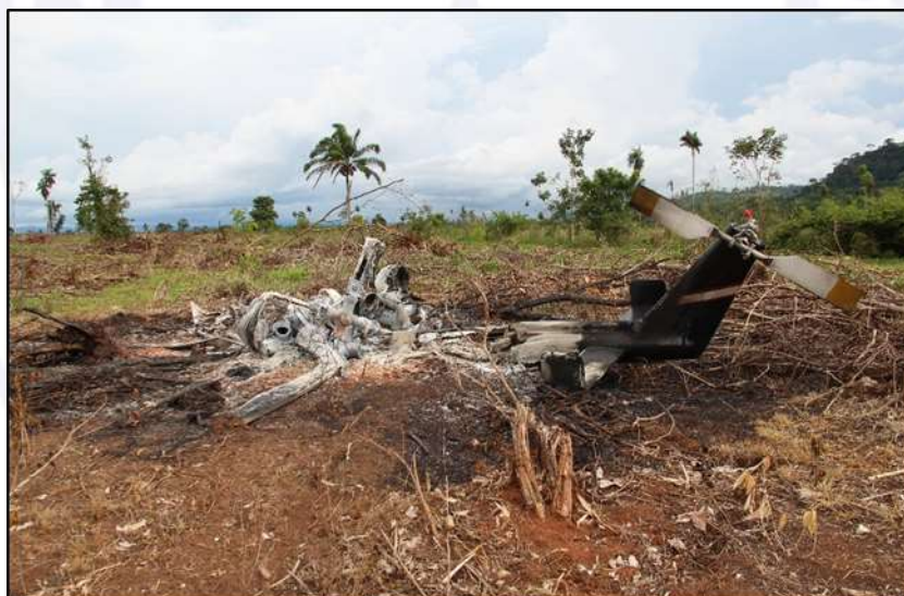
Figure 1 - Aircraft after being consumed by fire.
