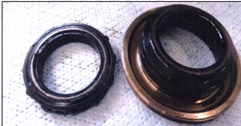
Figure 9 – Overview of the engine power turbine rear bearing.
