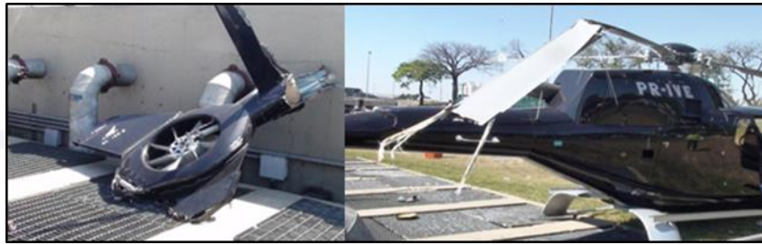
Figure 2 - View of the fenestron and the main rotor sectioned.
