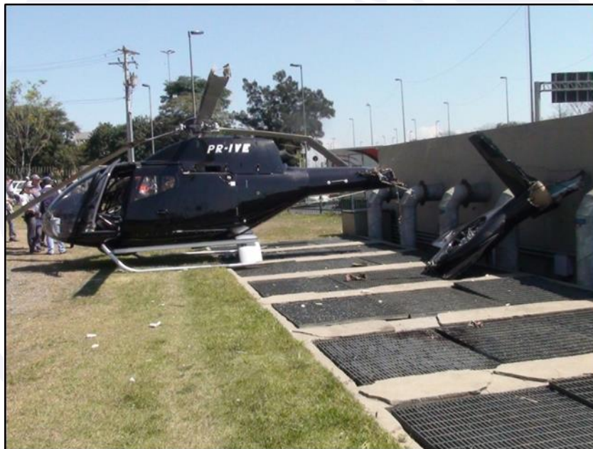
Figure 1 - View of the aircraft after the collision against a concrete wall.
