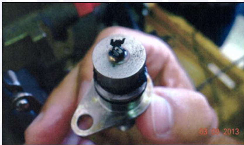
Figure 4 - Magnetic Plug of the M01 with particles.
