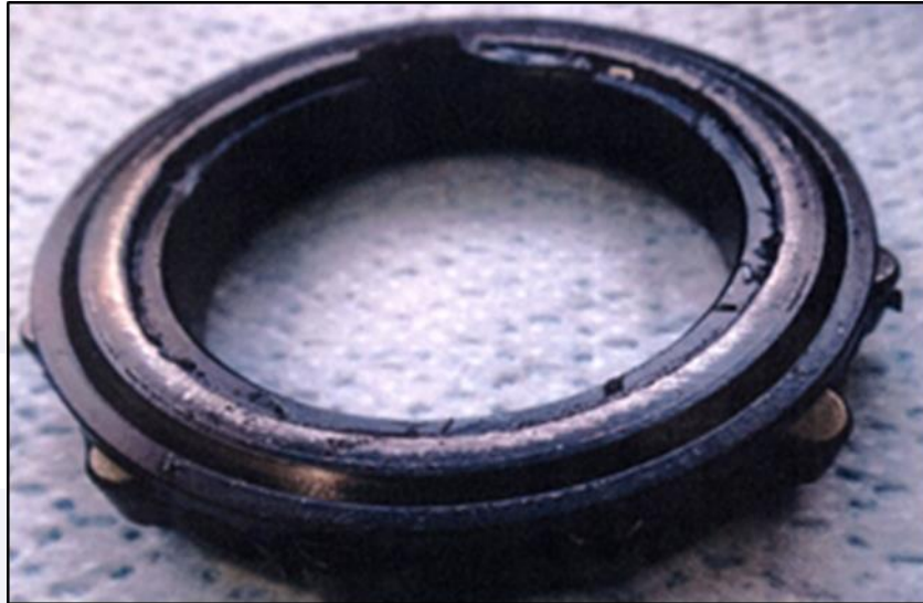
Figure 8 - General view of the rear bearing of the gas generator.
