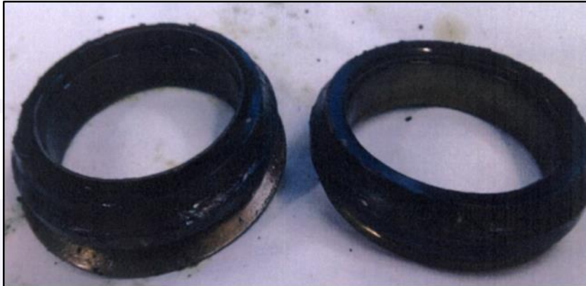
Figure 6 - M02 front bearing roller tracks with differentiated coloration in the track contact region.
