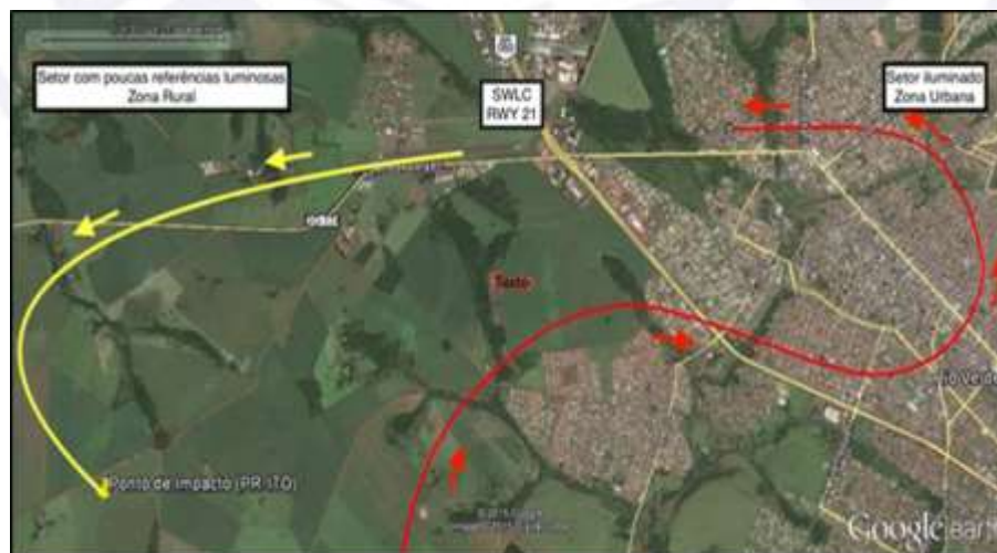
Figure 6 - Reconstruction of the aircraft traffic circuit recorded in the on-board GPS (in red) and the probable trajectory of the aircraft after the go-around procedure (in yellow).
