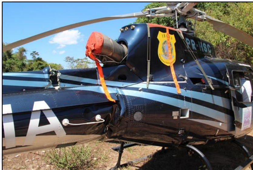
Figure 1 - Tail cone and fairing of the tail rotor drive shaft damaged.
