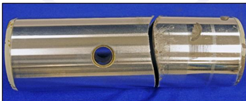
Figure 4 - Aft trunnion pin fractured.
