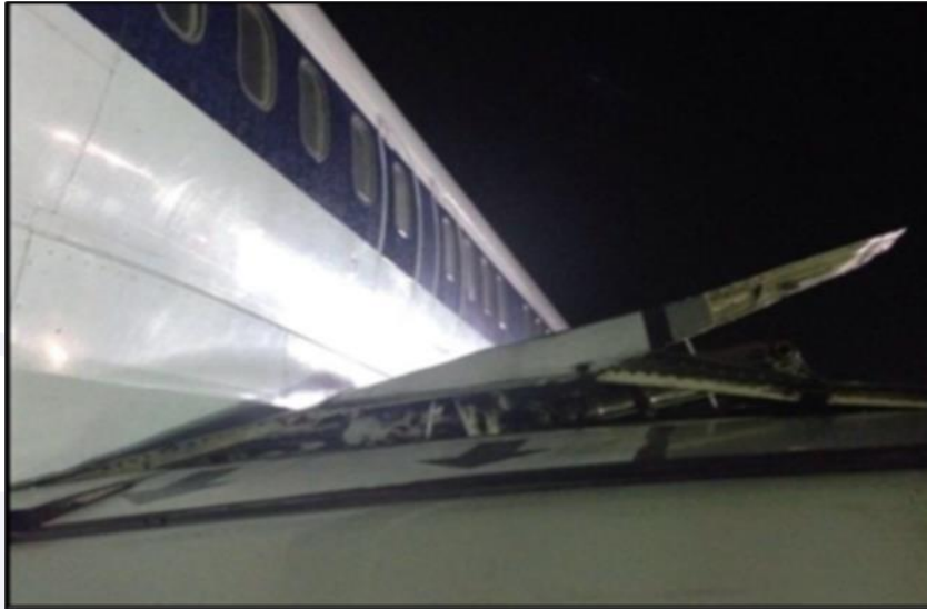
Figure 38 - Damage caused to the right wing's upper surface of the VT-JGD aircraft as a result of the break of the aft trunnion pin.
