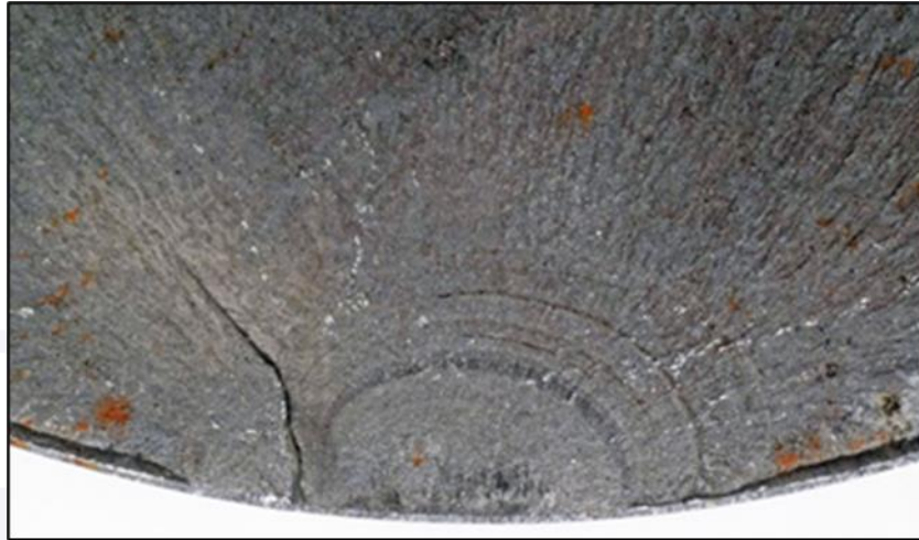
Figure 20 - Detail of the part 2 fracture of the aft trunnion pin.
