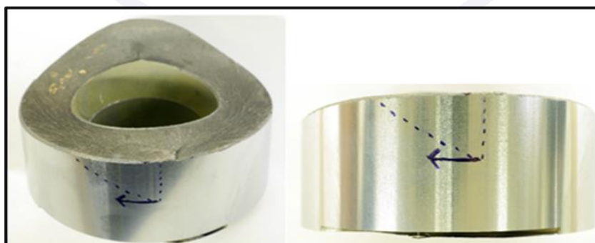
Figure 28 - Cut performed for metallographic examinations.
