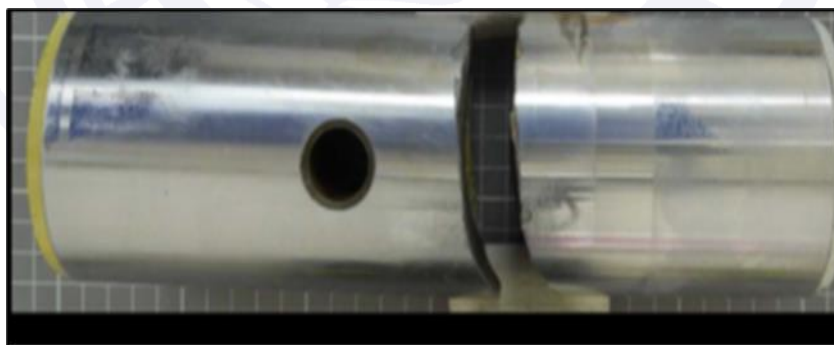
Figure 37 - Detail of the fractured aft trunnion pin SN 2430 that was installed on the right landing gear of the VT-JGD aircraft.
