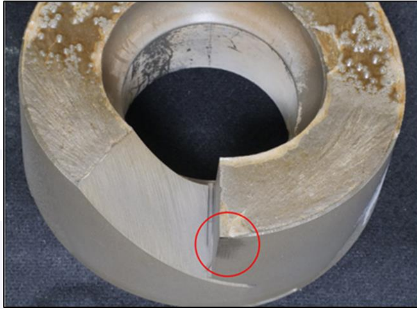
Figure 30 - Result of the inspection with Nital-Etch.
