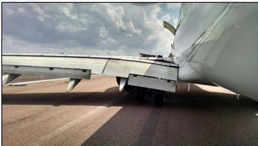
Figure 35 - Damage to the wing of the VT-JGA aircraft after the break of the aft trunnion pin.
