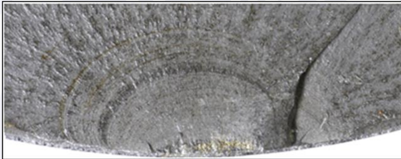
Figure 18 - Detail of the part 1 fracture of the aft trunnion pin.
