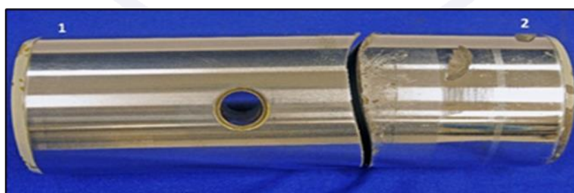
Figure 16 - Aft trunnion pin fractured.
