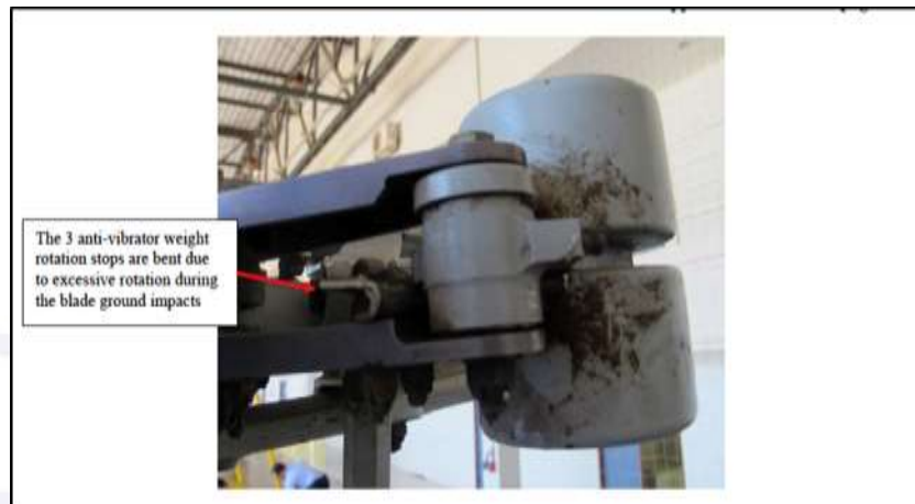
Figure 14 - Shock absorbers twisted, due to ground impact.
