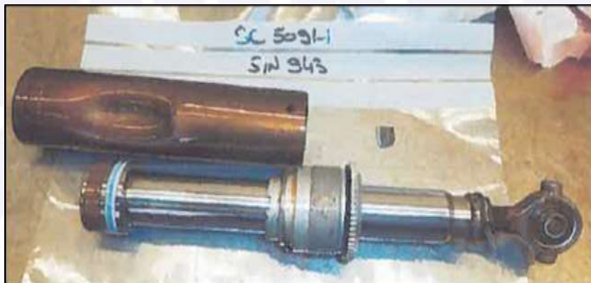
Figure 45 - Deformation of the S/N 943 servocontrol protection, due to the overpressure generated on the impact.
