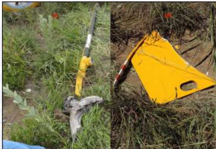
Figure 5 - (I) Left ski broken and disconnected. (II) Fenestron tail rotor guard disconnected from the aircraft.
