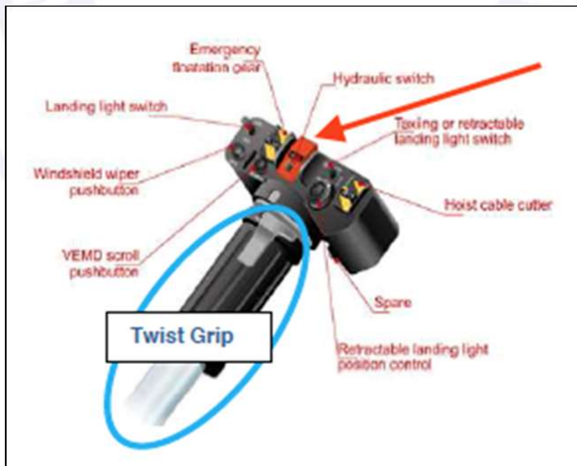
Figure 55 – Hydraulic Switch of the Collective Command.
