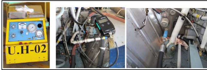
Figure 40 - Hydraulic bench connected in the crashed aircraft.
