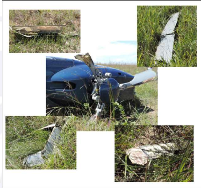
Figure 7 - Fragments of blades scattered on the wreckage site.
