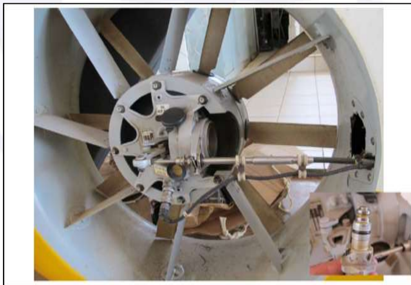
Figure 26 - Tail rotor and magnetic plug with no particles (highlighted).
