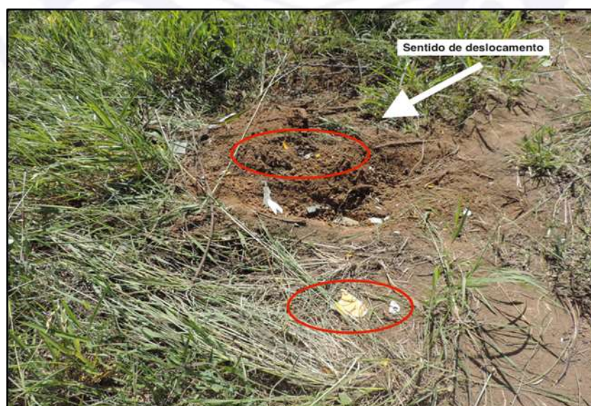
Figure 3 - First impact. In highlight, yellow ski ink and pieces of the fenestron-type tail rotor guard.
