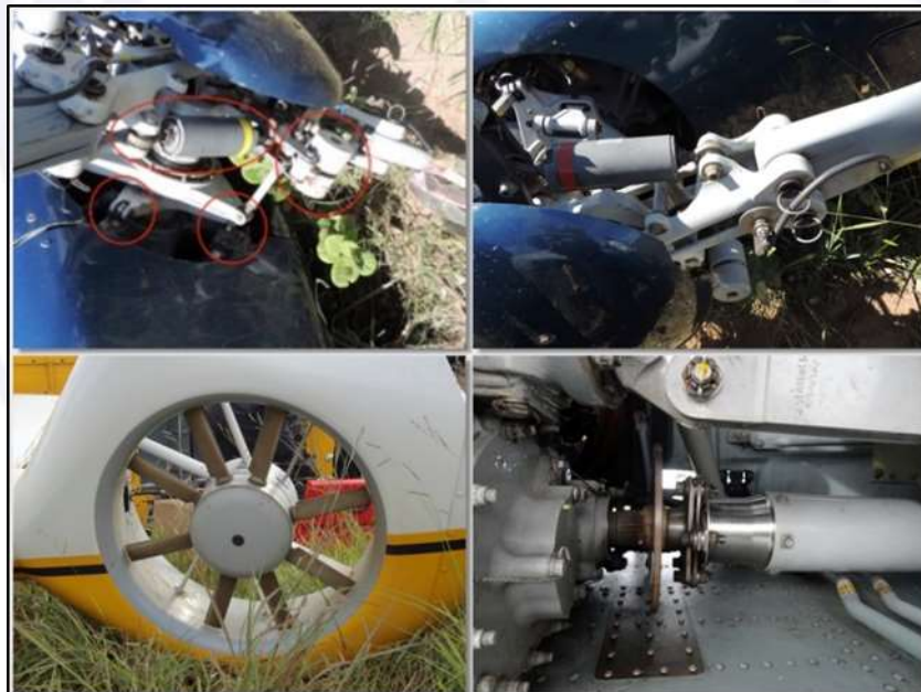
Figure 8 - Rotor head and its connections, vibration absorbers, fenestron rotor and engine connection shaft.
