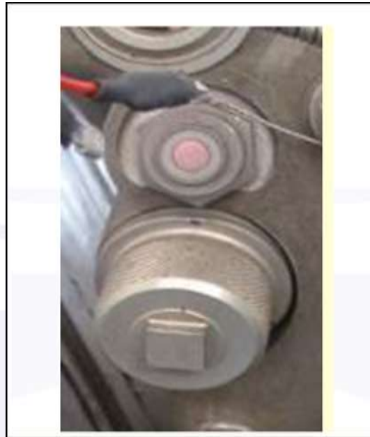
Figure 38 - Hydraulic filter indicator not triggered.
