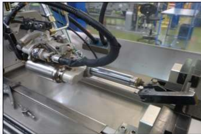
Figure 43 - Functional test in the servocontrols.
