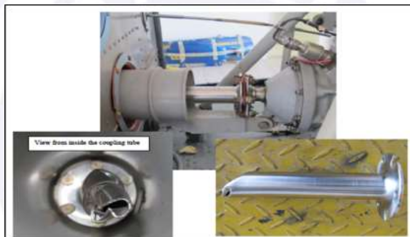
Figure 20 - Internal view of the coupling tube and broken drive shaft.
