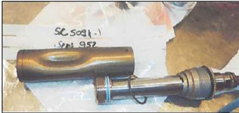
Figure 44 - Deformation of the S/N 952 servocontrol protection, due to the overpressure generated on the impact.
