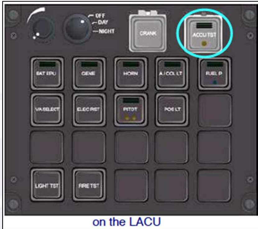
Figure 53 - ACCU TST on the LACU (Light and Auxiliary Control Unit).
