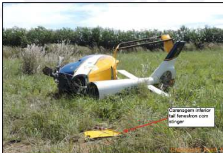
Figure 6 - The lower protection fennel shield was disconnected.
