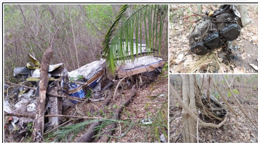
Figure 4 - Fuselage resting on back and separate engines.
