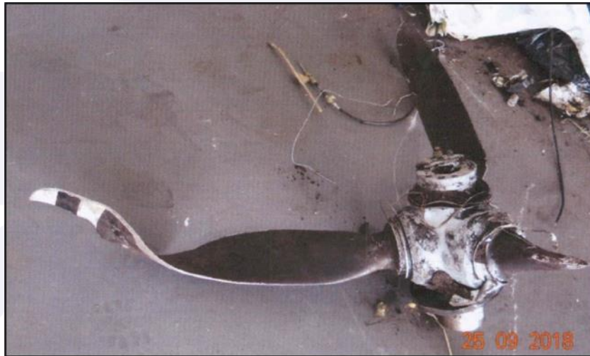
Figure 11 - Detail of fractures and deformations in the three propeller blades of the left engine.
