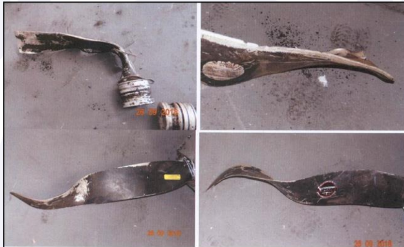
Figure 13 - View of the right propeller blades with forward-facing folds.
