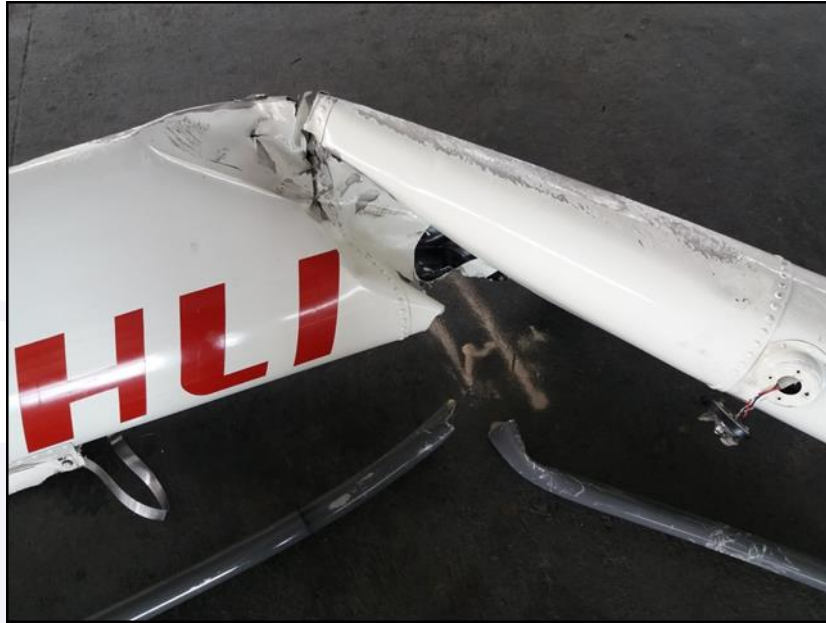
Figure 20 - Tailcone bents, due to impact of the main rotor blade.
