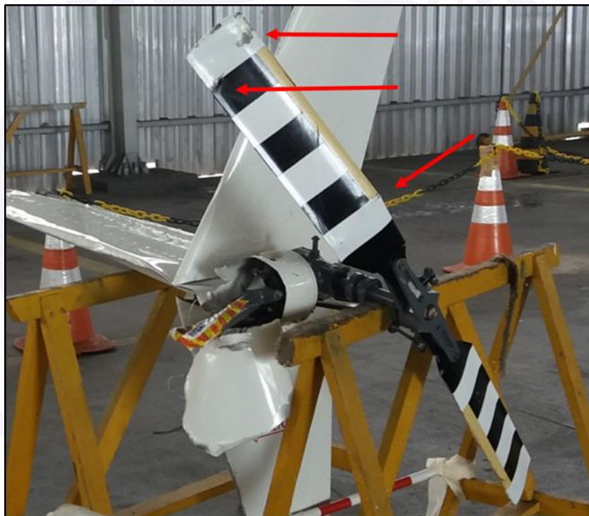
Figure 21 - Damage to the tail rotor blades highlighted by red arrows.
