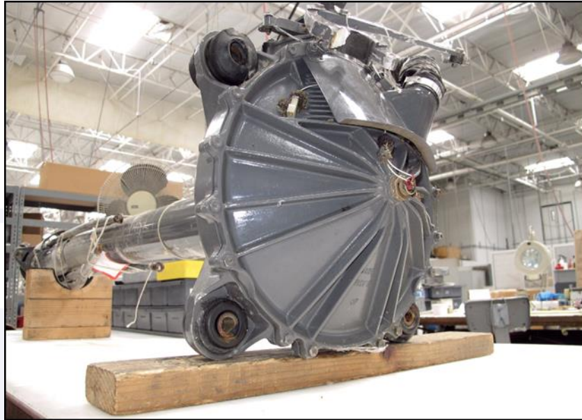
Figure 23 - General appearance of the MGB before disassembly.
