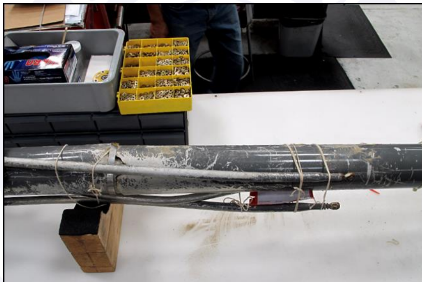
Figure 24 - Damage to external mast fairing.
