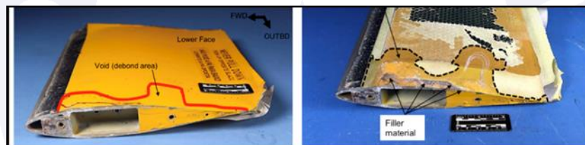
Figure 46 - Bottom surface of the blue blade (S/N 6131) in two moments: Left, after the tap test; and on the right, after removing the lower skin. (Source: Adapted from NTSB).
