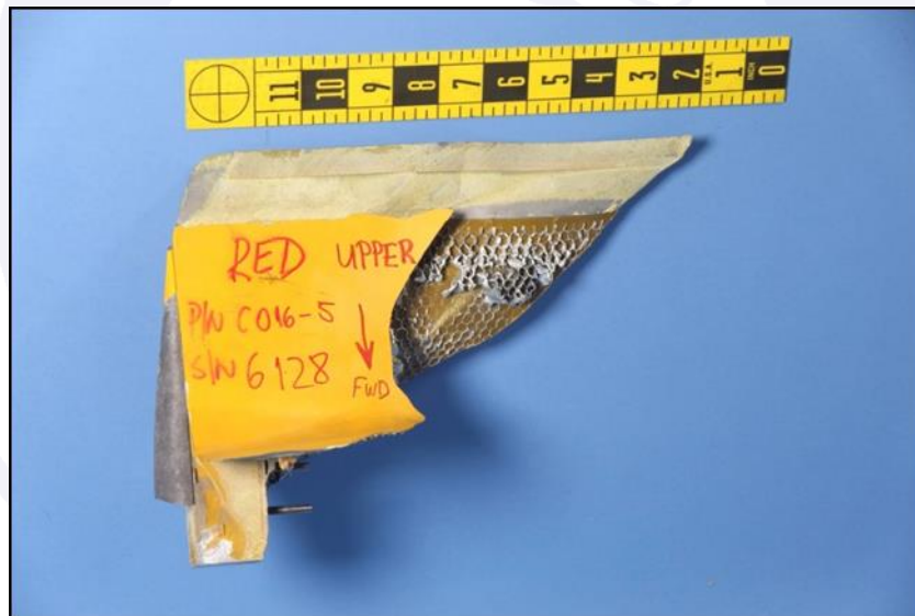
Figure 27 - Red blade fragment (S / N 6128) sent for laboratory tests. (Source: Adapted from NTSB).
