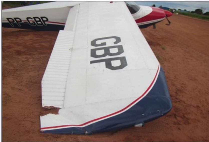
Figure 3 - View of the right wing damage.
