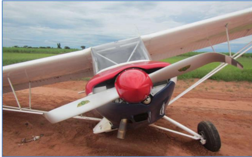
Figure 2 - View of the damage to the propeller blades and landing gear.
