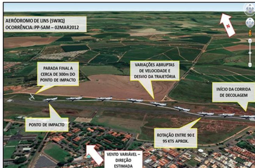
Figure 3 - Sketch of the occurrence, from the take-off to the final stop (out of scale).
