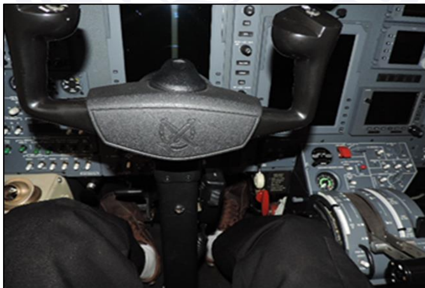
Figure 15 – View of the panel for the pilot positioned on the left seat of the Cessna 525. The stick column obstructs the view of the emergency brake actuator handle.
