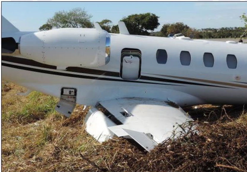
Figure 11 - Flaps configuration in 60° and open speed brake - right wing.
