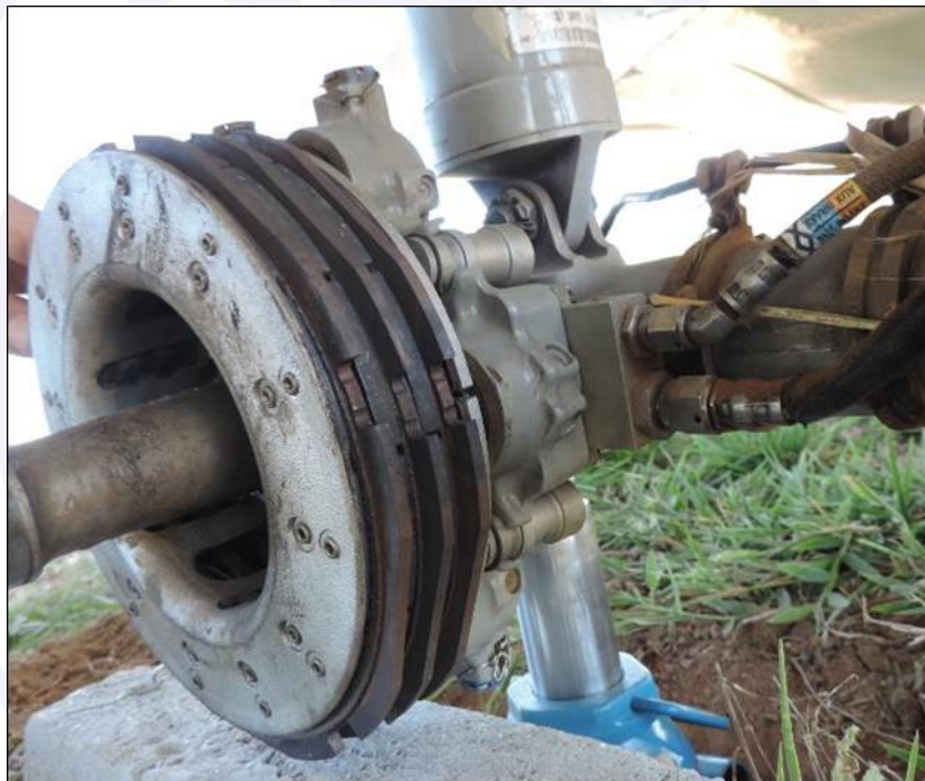
Figure 20 - Right brake assembly and hydraulic and pneumatic power lines.
