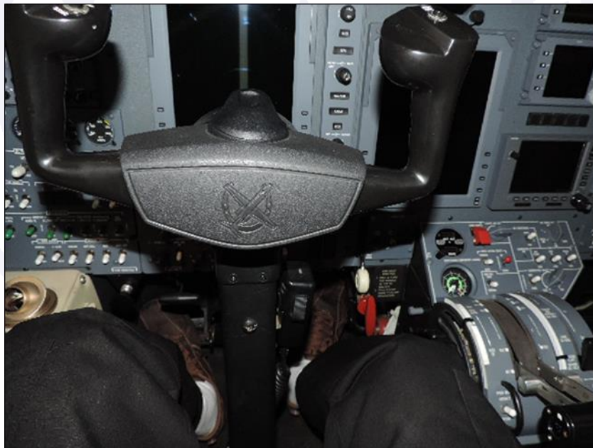
Figure 15 – View of the panel for the pilot positioned on the left seat of the Cessna 525. The stick column obstructs the view of the emergency brake handle.
