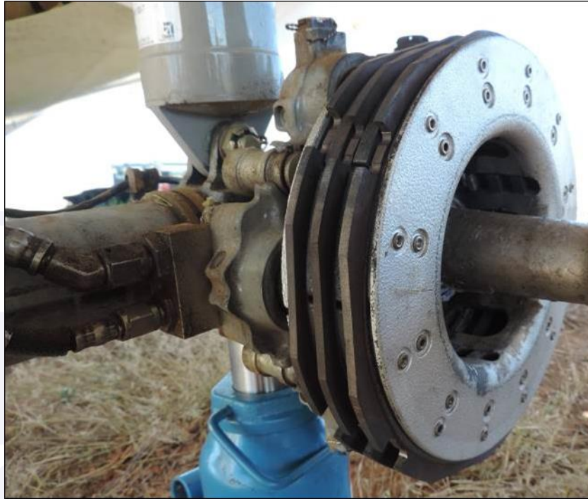
Figure 19 - Left brake assembly and hydraulic and pneumatic power lines.
