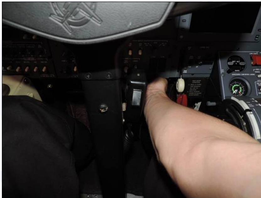
Figure 17 - Simulation of the emergency brake lever drive.
