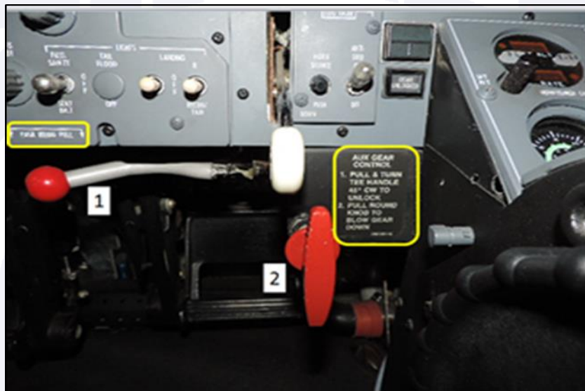
Figure 27 - Panel of the 525. (1) - emergency brake actuator handle, with the description EMERG BREAK PULL, highlighted in yellow in the photo; (2) - auxiliary gear control, with the description AUX GEAR CONTROL.
