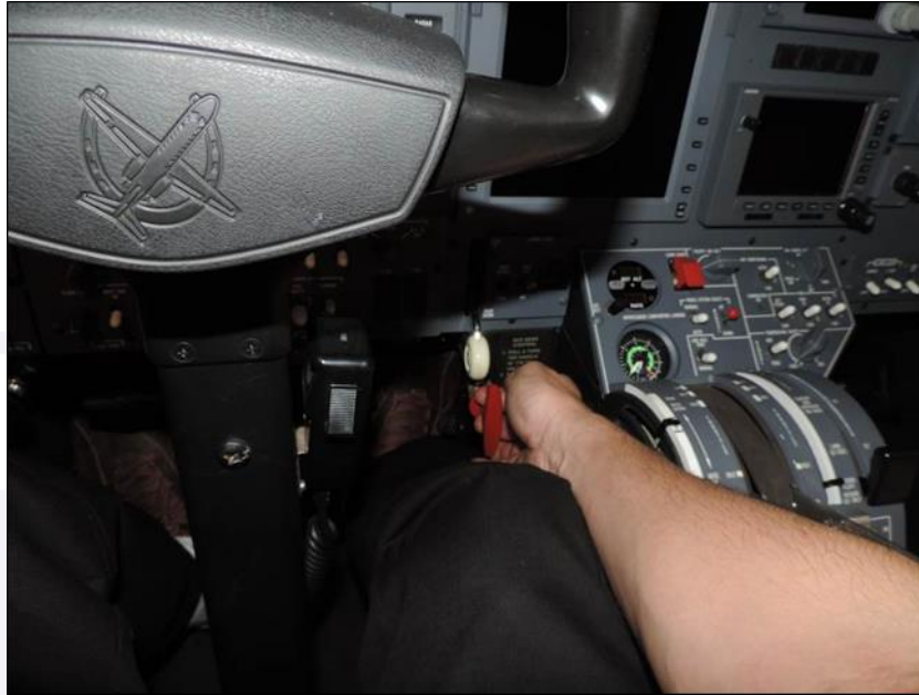
Figure 16 - Visualization of the emergency landing gear lever by the pilot positioned on the left seat.
