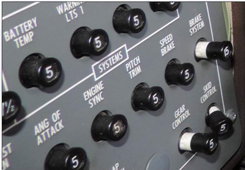
Figure 9 - Disarmed circuit breakers - BRAKE SYSTEM, GEAR CONTROL and SKID CONTROL (SYSTEMS).
