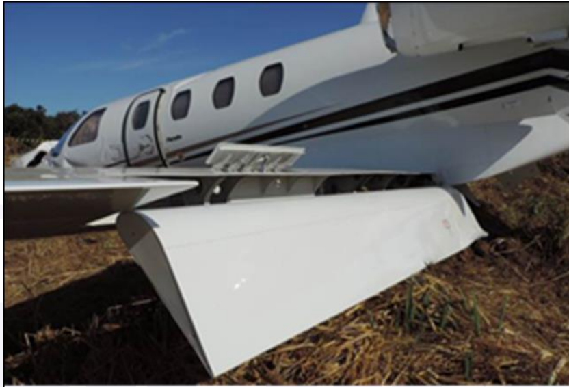
Figure 10 - Flaps configuration in 60° and open speed brake - left wing.
