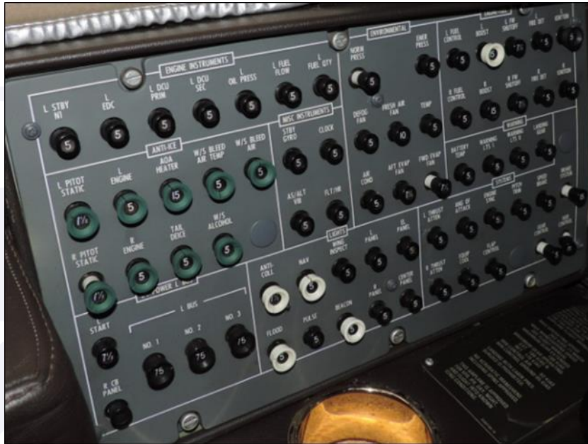
Figure 8 - Left circuit breaker panel.
