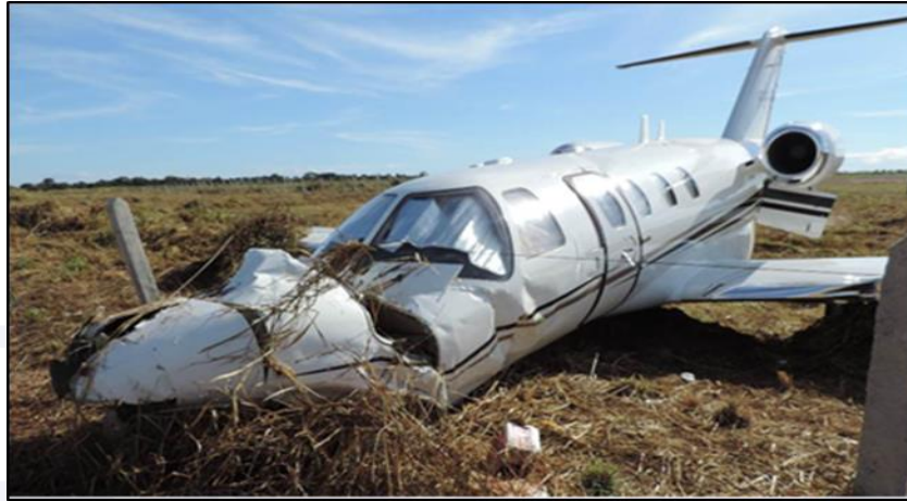
Figure 5 - Damage to the front section of the aircraft.
