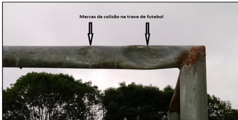
Figure 1 - Marks from the collision of the tail rotor blades against the soccer goalpost.
